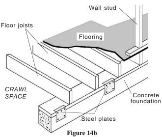
**Figure 14**—Anchor bolts or steel plates. A home's crawl space may be formed by a cripple wall (*see next page for description*) between the foundation and the floor joists or the floor joists may rest directly on the sill plate. In either case, you should be able to see the heads of anchor bolts or steel plates installed at appropriate intervals. These fixtures fasten the sill plate to the foundation.
