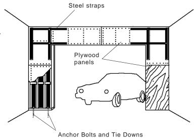
**Figure 32—Bracing garage walls.** If your house has a room over the garage, the garage walls may not be strong enough to hold up during an earthquake unless they are braced with plywood panels and steel straps.
