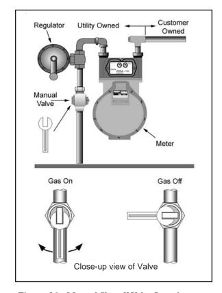
Figure 36—Manual Shutoff Valve Location
